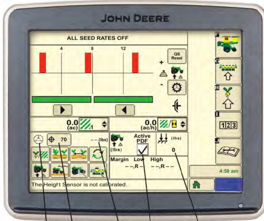
Active PDF status Target margin Actual margin Active system on/off check box Actual down force in air spring circuit
